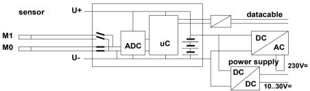
he analog inputs are electrically isolated by means of photovoltaic relays; the maximum potential difference permitted between them is 50 VDC or 60 VAC. The power supply is isolated by the transformer in the mains adapter or by a DC/DC converter in connecting cable ZA2690-UK.
