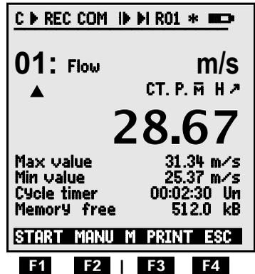
**Measuring point selection** by means of cursor keys (3) (M in the middle)
