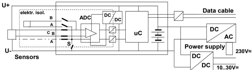
The analog inputs are electrically isolated from one another by means of photovoltaic relays. A new feature on this device is the additional separation of the measuring inputs from the CPU and power supply. Between all inputs and outputs (even the analog output cables which are not electrically isolated) the maximum potential difference permitted is 50 V. The voltage at the measuring inputs themselves must not exceed 12 V (between B, C, D, and A).
